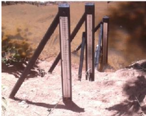
Figure 18: Linimetric Section and automatic level sensor
