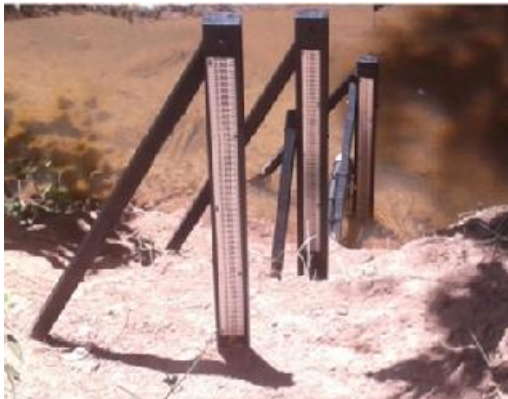
Figure 18: Limimetric Section and automatic level sensor
