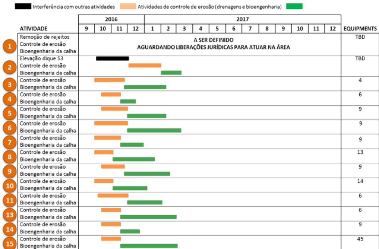
Figure 39: Schedule of activities of reconfiguration of the river channels and erosion control
